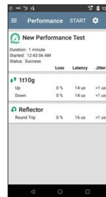
Performance test with up to 4 streams and 4 end points
