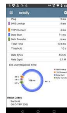
HTTP test reveals cloud/web-based services response times
