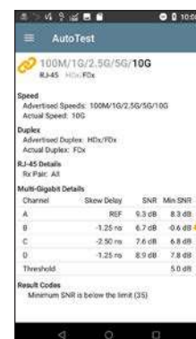
Cabling SNR measurement validates Multi-Gig links
