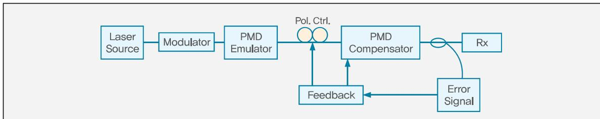
**(3) FEC (Forward Error Correction) Performance Test against PMD stress**
