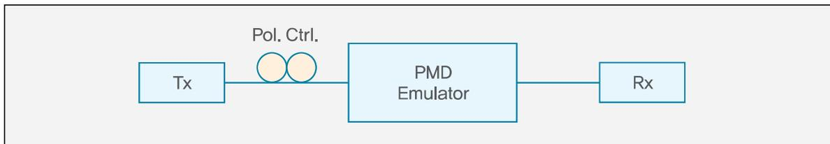
**(2) PMD Emulations for testing PMD Compensator / PMD Compensation experiment**
