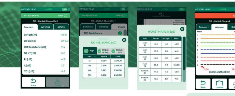
TestPro supports testing and certification for network deployments up to 40 Gigabit Ethernet for Cat 5e, 6, 6A, 7, 8 or Class I/II cabling system. The electrically centered test plug assures the Level 2G/VI accuracy required to support field testing to Cat 8 / Class I/II, and actually exceeds the 2000 MHz requirement, to offer a 3000 MHz platform. As a result, you can feel confident in results over the full frequency range.
