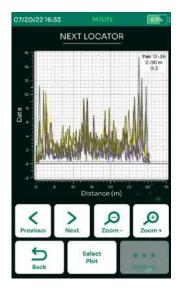
TestPro offers fault location for Return Loss, NEXT, and Shield aiding in problem identification. Support for MPTL, Patch Cord, Single Pair, GG45, Tera, and Coax is available through hot swappable adapters. At the completion of the Autotest, you get a highly visible Pass or Fail indication, and test results can be automatically saved with a customizable labeling scheme.
