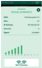
Useful for moves/adds/changes as well as general troubleshooting, TestPro will connect to a live network through the AD-NETCABLE adapter, or wireless using the optional Edimax Wi-Fi USB adapter.
