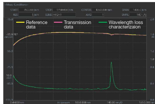
Measurement example of wavelength loss characterization with AQ6374E
