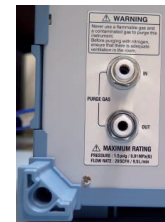
Purge gas ports (input and output)
