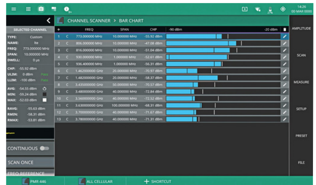
Bar Chart Display Monitoring GSM, LTE, and 5G Cellular Bands
