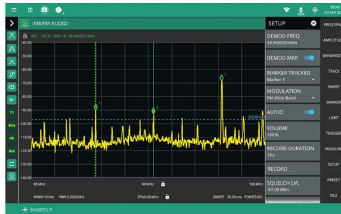
AM/FM Signal Demodulation at Marker Frequency
