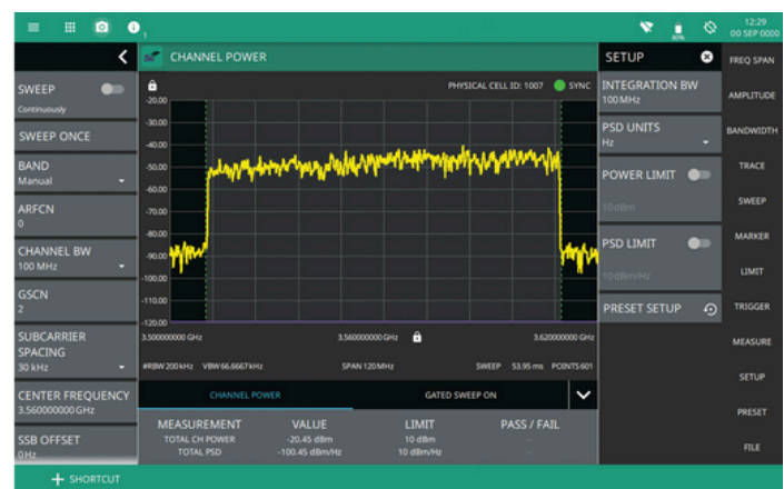
5G Channel Power Results in 5G Mode
