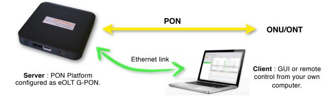
The **eOLT G-PON** license allows to configure and use the **PON Platform**, our high performance FPGA-based processing unit (see corresponding datasheet), as an G-PON eOLT emulator kernel. The GPON eOLT kernel is controlled from a dedicated eOLT client GUI software installed on a regular PC. MT2 eOLT G-PON's architecture stems from our reference GPON OLT emulator, which is at the core of LAN's BBF.247 official certification testbed, and shares its key features:
