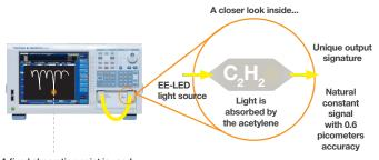
A fixed absorption point is used to re-adjust the internal calibration table
