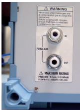
Purge gas ports (input and output)
