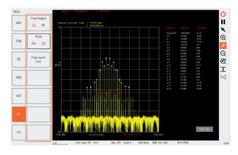
The new BOSA 400 series can be made possible only thanks to the high quality components inside and the careful control of all of them. Besides, all the graphic interface has been redesigned to be faster and more operative than ever. Take most of your measurements with some of the advanced functions:
