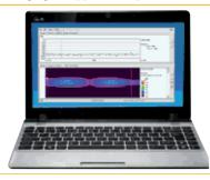
In Spectrogram mode ET 92 performs spectrum measurements in every second. The results are directly transferred to PC via USB port or indirectly by means of a memory stick when the measurement is completed.
