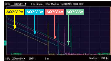
Trace examples with pulse width of 1 \mu s
