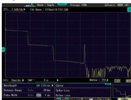
Example of measuring 128-port splitter with high SNR (HSN) mode
