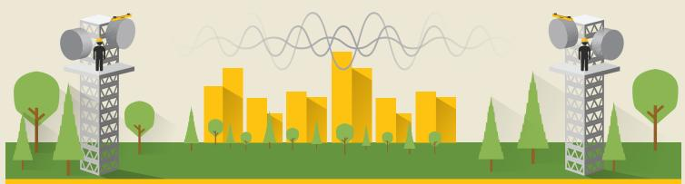
The system automatically calculates exact alignment using known positional data in real-time and provides the user simple targets for aligning the link. No signal, power, or frequency is needed for Sunsight's innovative patented pathing process.
