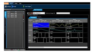
In the Multi-sequence mode, two sequences can be defined to control Channel 1 and Channel 2 (and the corresponding digital channels) separately as two units of generator.
