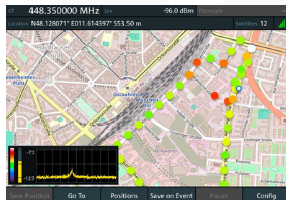
Coverage measurements via level mapping with integrated spectrum view.
