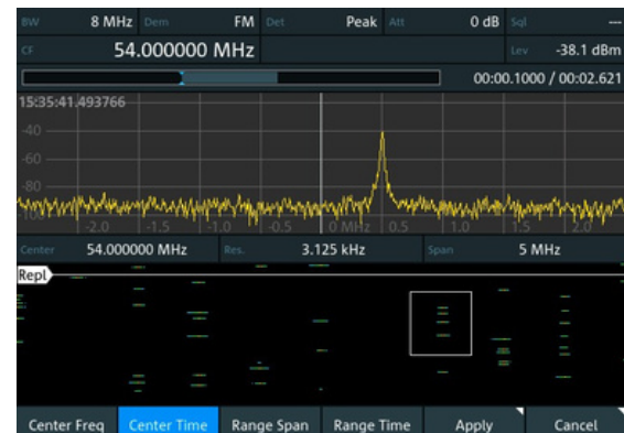
Detailed display of spectral signal characteristics with increased time resolution.
