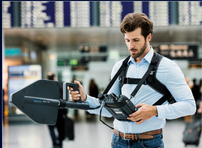
Manual homing direction finding with the R&S®PR200 and the R&S®HE400.
