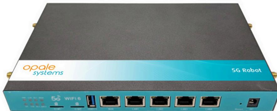
The Opale 5G Mobile Robot is a compact and versatile telecom Probe which supports 3G, 4G, 5G connectivity. Opale 5G Robot is ideal for bringing Mobile connectivity to any test application or to automate recurrent tasks on a mobile network.
