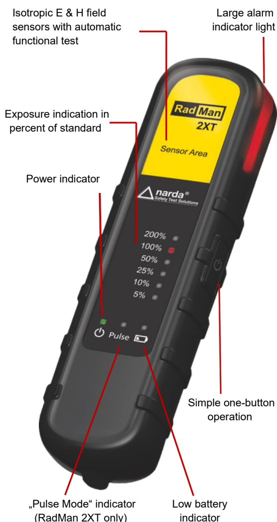
Fig. 1. Front view with controls and indicators
