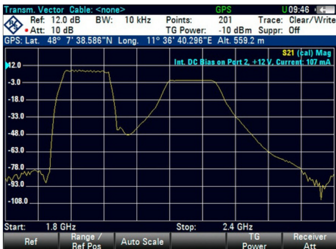
TMA transmission measurement: built-in voltage supply, current measurement with R&S®HA-Z240 GPS receiver connected
