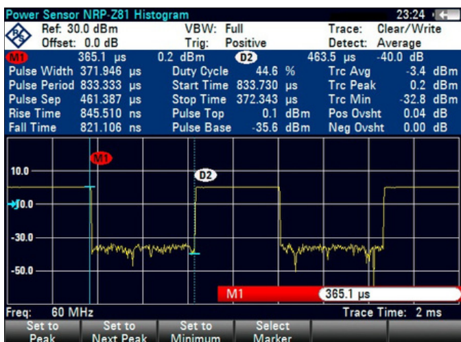
Pulse analysis with R&S®ZVH-K29 and R&S®NRP-Z81 wideband power sensors
