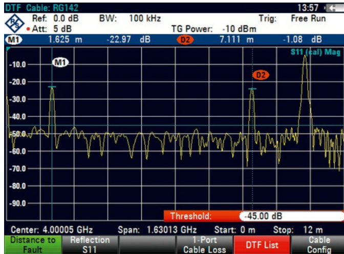
Distance-to-fault (DTF) measurement
