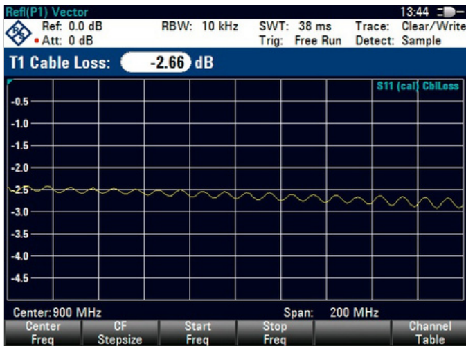
One-port cable loss measurement
