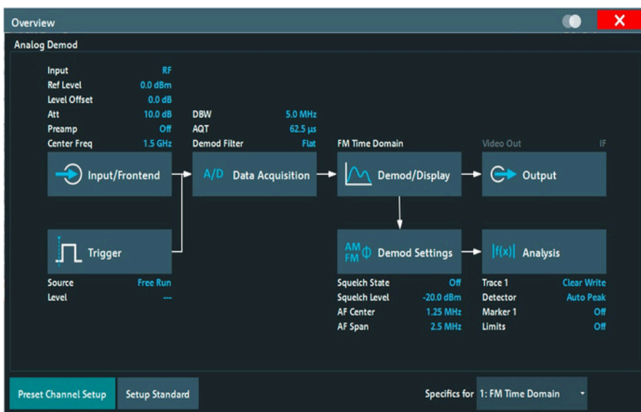
Overview of analog demodulation menu: all setting functions are accessible here.
