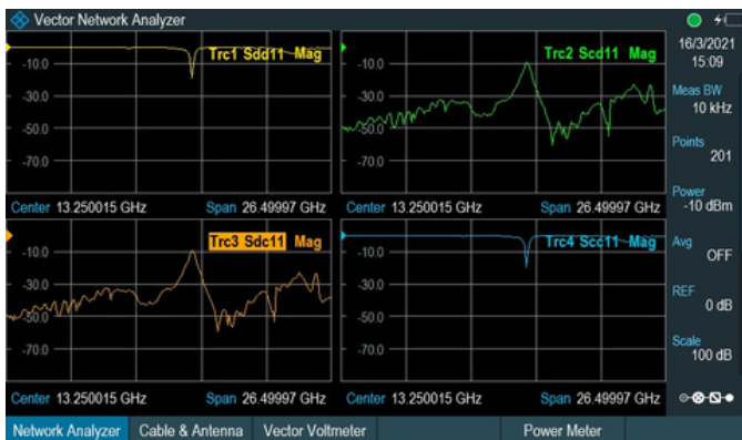
R&S®ZNH-K47 mixed mode measurement.
