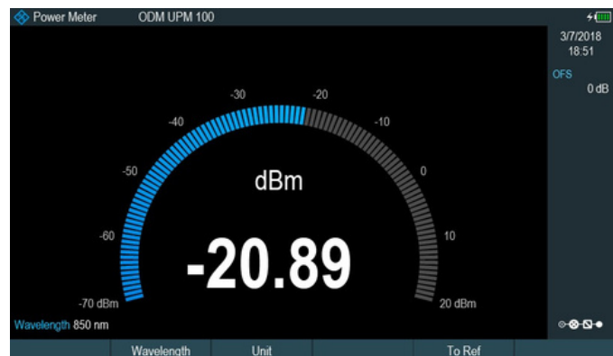
Optical power measurement with optical power sensor.
